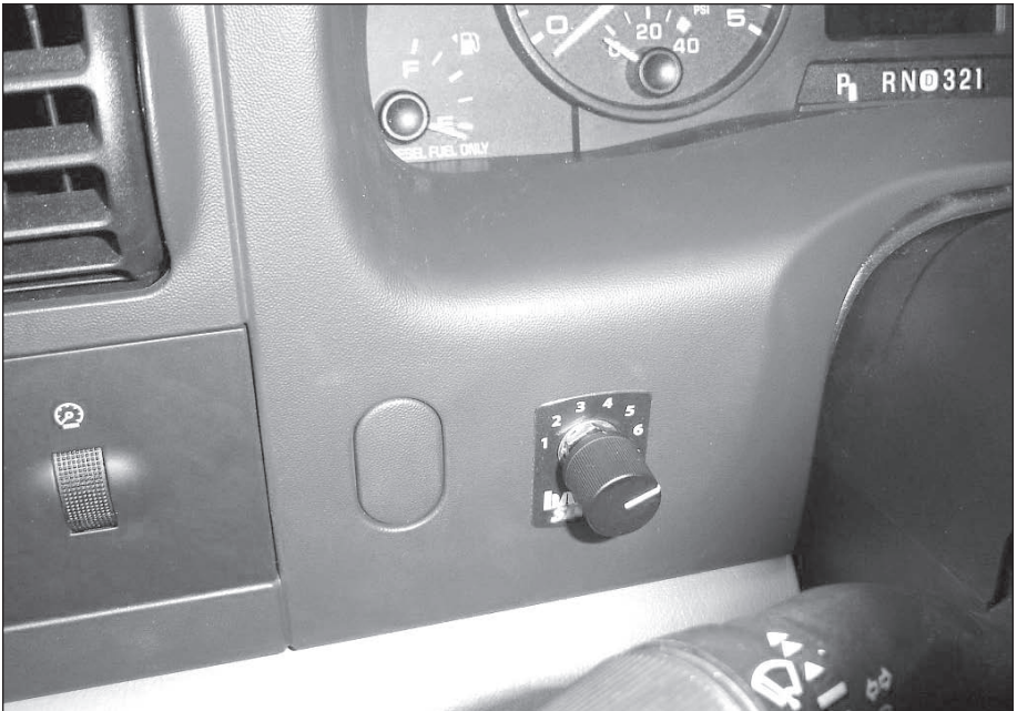
Figure 15a Finished installation of the Six-Gun switch on 2005-06 model year vehicle
