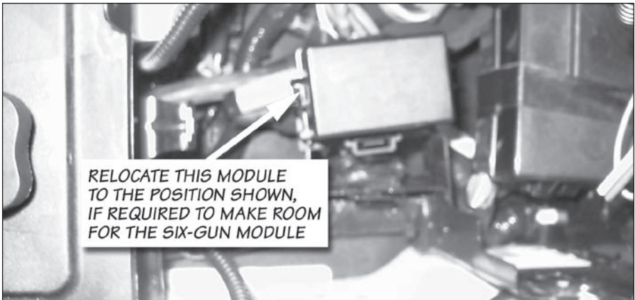
Figure 9 Electronics module to relocate on 4-wheel-drive vehicles (2003-04 model year vehicles only)
