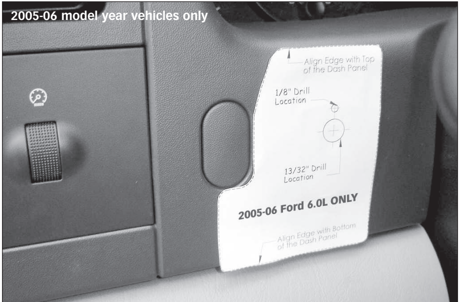
Figure 13a Template taped to front of dash on 2005-06 model year vehicle, ready to be drilled.
