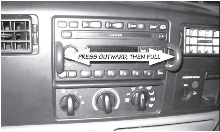
Figure 11 Removal of the stereo (2003-04 model year vehicles only)
