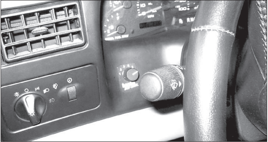
Figure 15a Finished installation of the Six-Gun switch on 2005-06 model year vehicle
