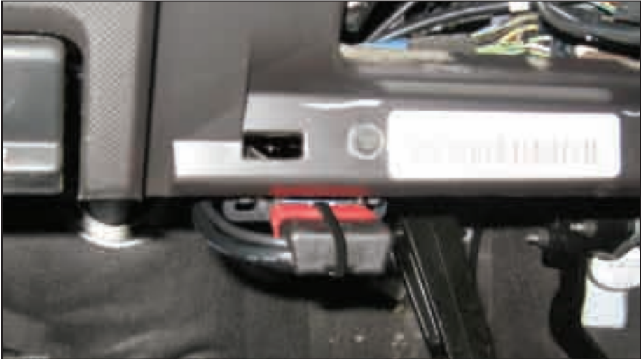
Figure 18 OBD II connection
