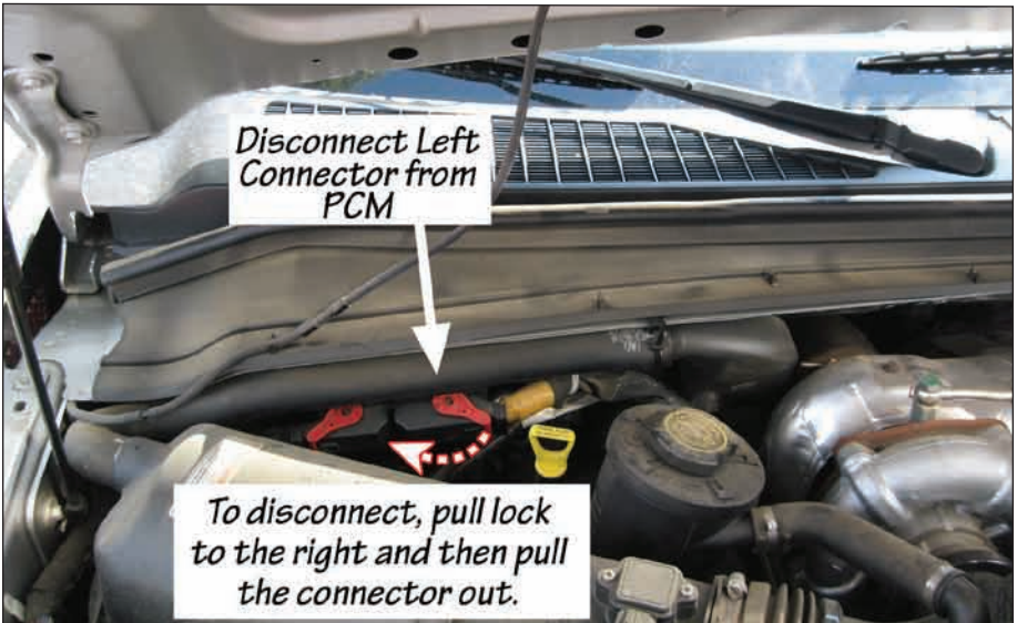
Figure 3: PCM Location on Passenger side.
