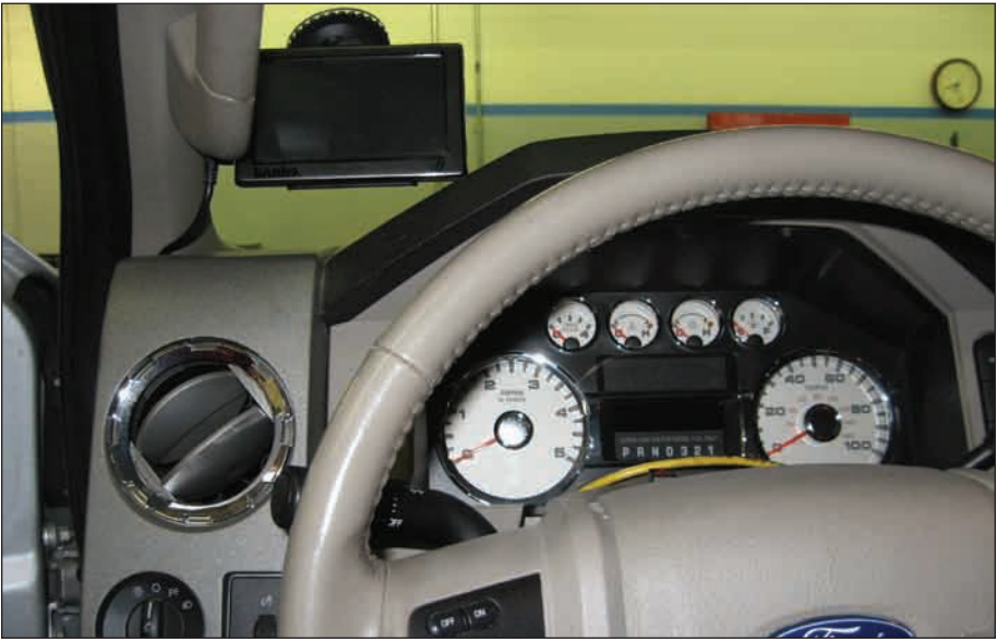
Figure 17 Suggested Mounting location for Banks iQ
