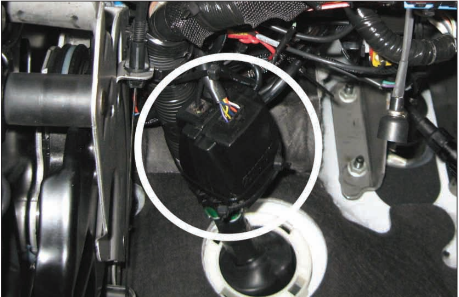
Figure 15 Banks Brake Module mounting location
