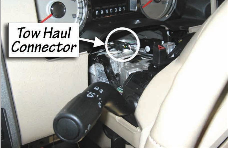
Figure 14 Tow Haul Connector on steering column, under main harness
