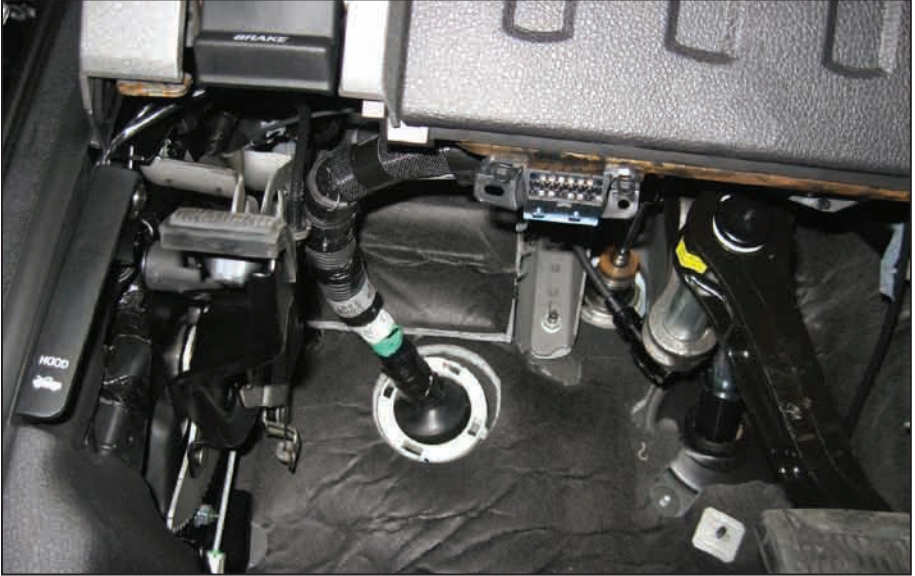
Figure 6: Rubber Grommet on driver side Fire wall
