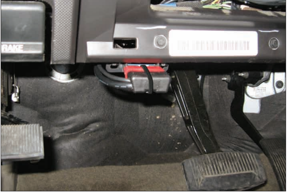
Figure 12 Brake Position Sensor location under dash
