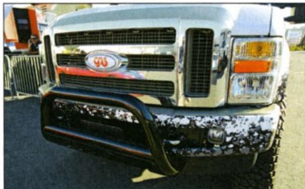
Since the new Ford trucks house seven radiators up front to cool various engine fluids, a Smittybilt Grille Saver was installed to protect them from off-road obstacles.
