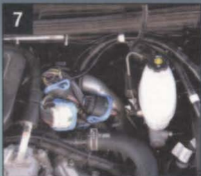
7 We cleaned the top of the fuse box and installed the SpeedBrake.
