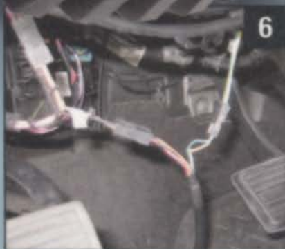
6 We connected the SpeedBrake cable to the PowerPDA harness.
