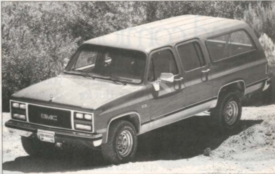
Both Chevrolet and GMC sell the Suburban, a vehicle unique among light trucks. The last competitor in the Suburban's class was the Travelall, and International Harvester stopped manufacturing it in 1975. We tested a GMC V-2500 Suburban equipped with the 6.2-liter diesel and optional Banks turbocharging system.
